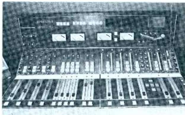
Figure 7 The WABC production control room 8C console, shown during installation, is used to make pre-recorded shows and promos.
